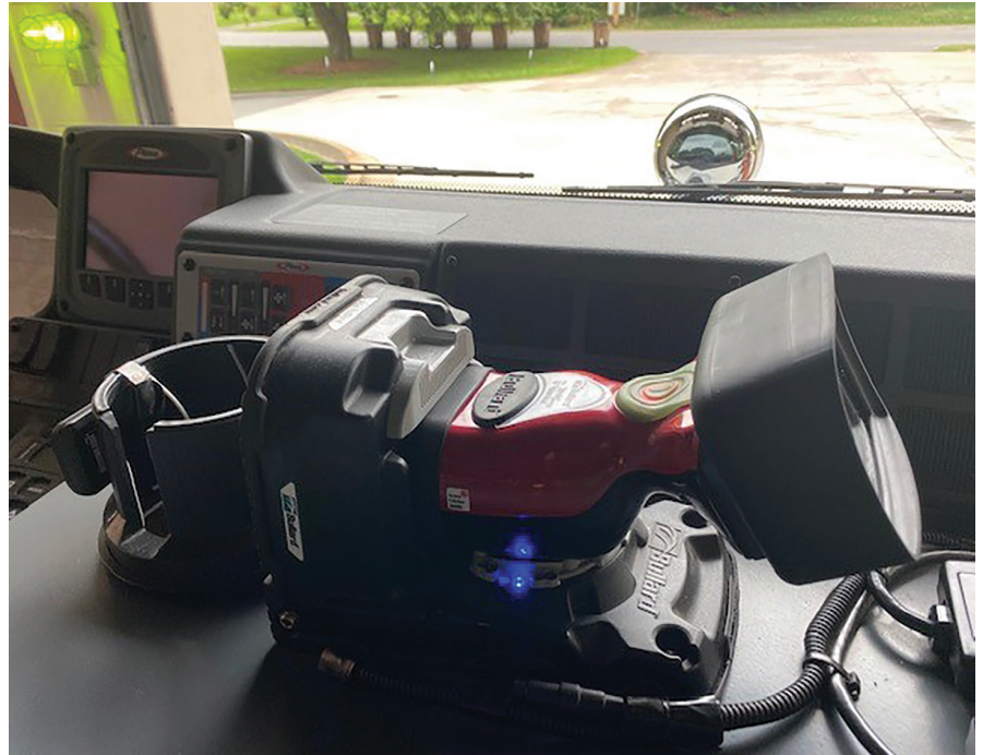
ABOVE: A thermal imager mounted in front at the officer's riding position.
