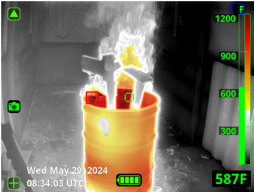
LEFT: Showing Low Gain state indicated by the green box with triangle in upper left corner. (Photo courtesy of Bullard.)
