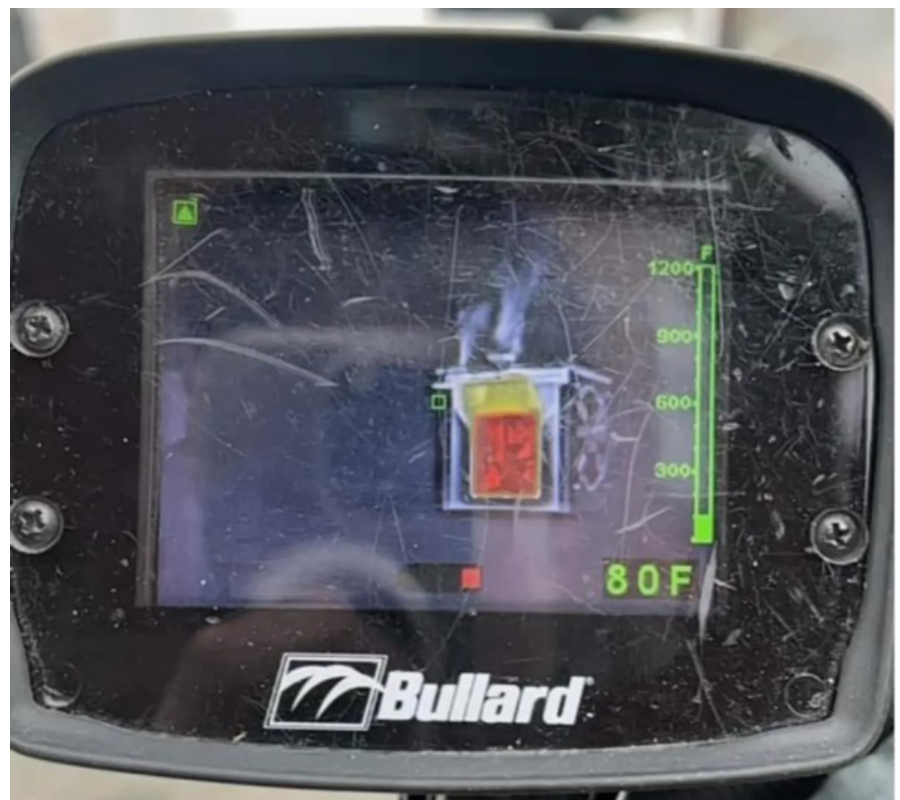
RIGHT: A scratched display screen that can be replaced in house. (Photo courtesy of Bullard.)
