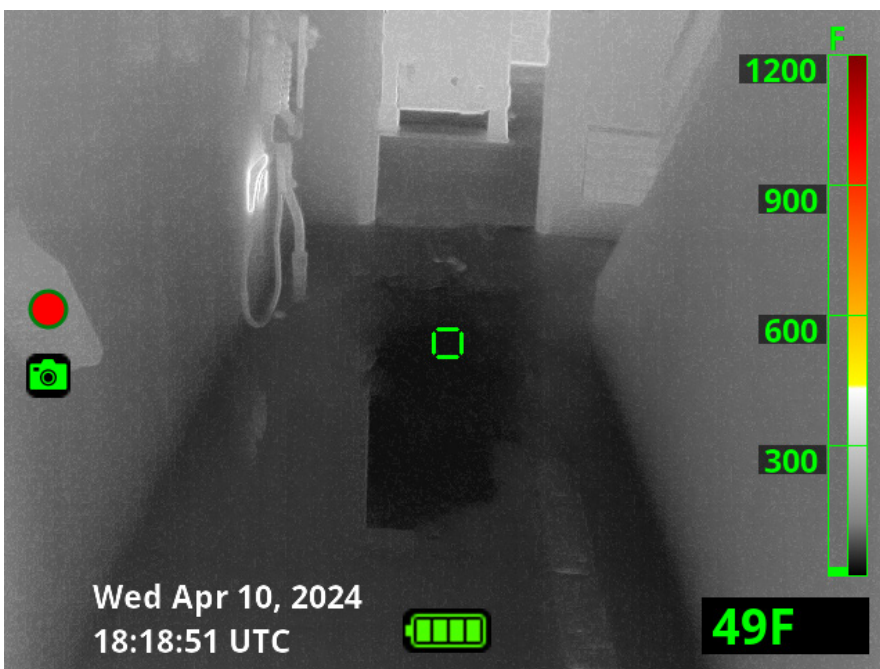
Above: Showing a hole in the floor or is it a reflection that looks like a hole. (Photo courtesy of Bullard.)
