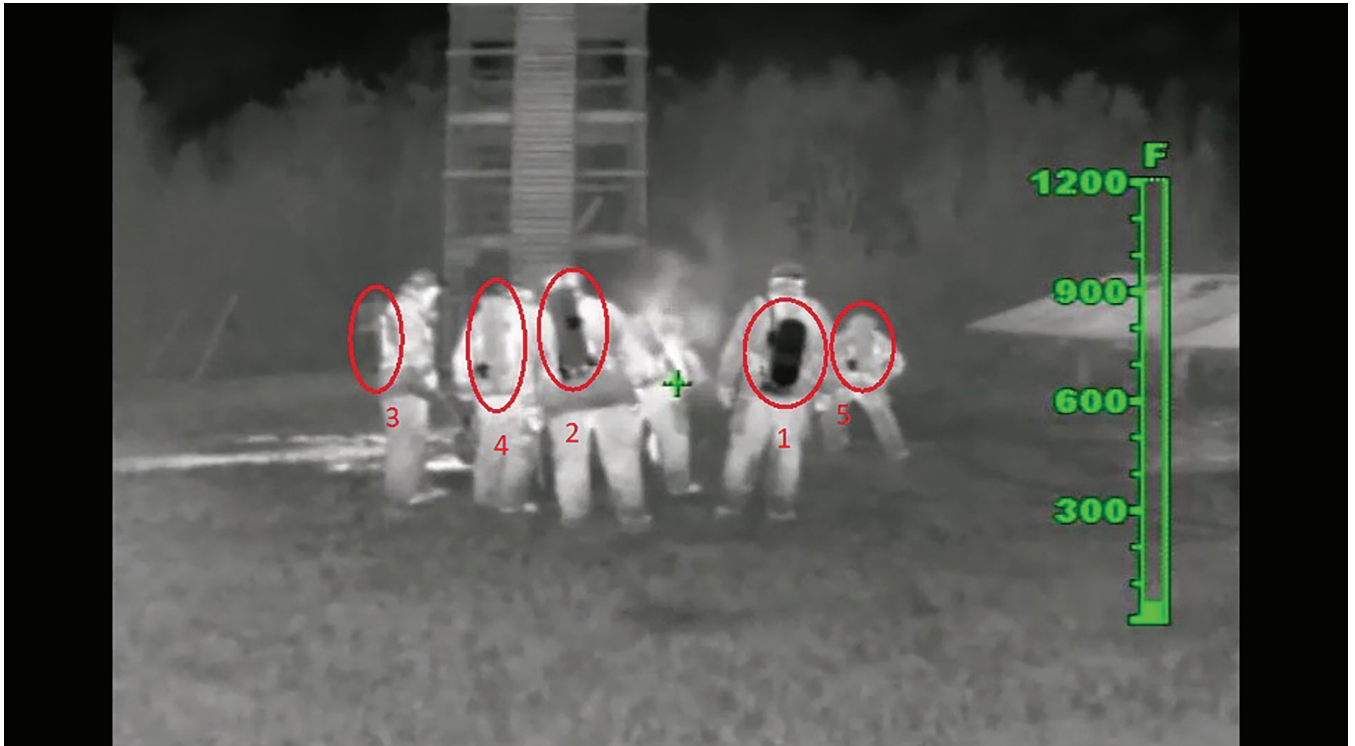
1. Five SCBA cylinders indicating different colors based on duration of use. (Photo courtesy of Bullard.)
