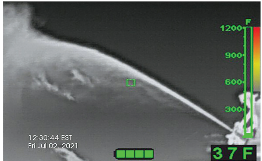
2. Monitoring a deck gun flowing water.
